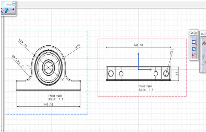
**Figure. Design of Bearing**
