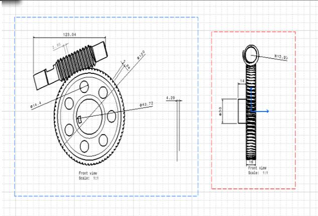
**Figure. Design of Worm Gear**
