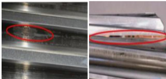
Fig. Examples of the local gear faulty problems
