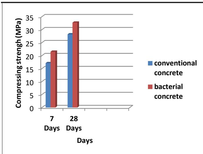
Graph 1- Compressive strength of conventional and bacterial concrete bloc at 7 & 28 days.
