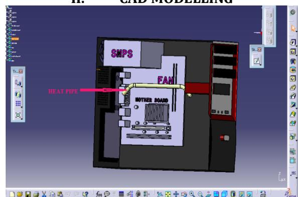
**Fig.2, CAD Model of CPU Heat Pipe.**
