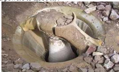
**Fig. 4 Gyratory crusher**
