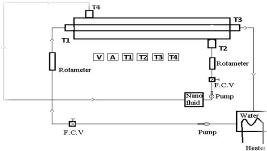
**Fig.5, Heat Exchanger**
