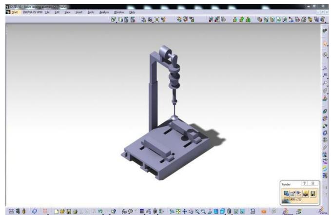
Figure 1.Valve Cleaning Machine 3D model
