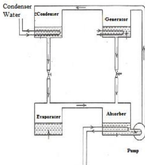
Fig. 3 Block diagram of VARs.
