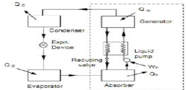
**Fig.2. vapour absorption cycle**
