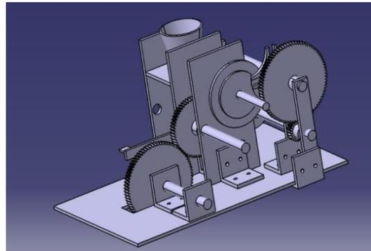
Fig.4 3D Model Of Seed Sowing Machine
