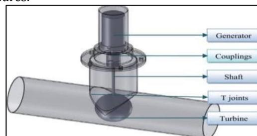
Fig.1: In-Pipe Turbine System Setup
