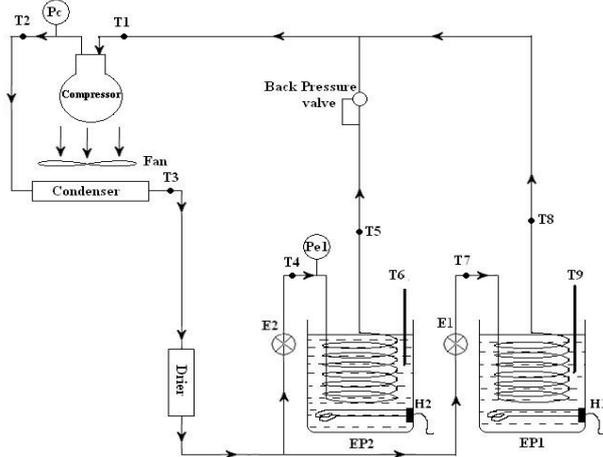
**Fig.1: Schematic Layout of the Experimental Setup**
