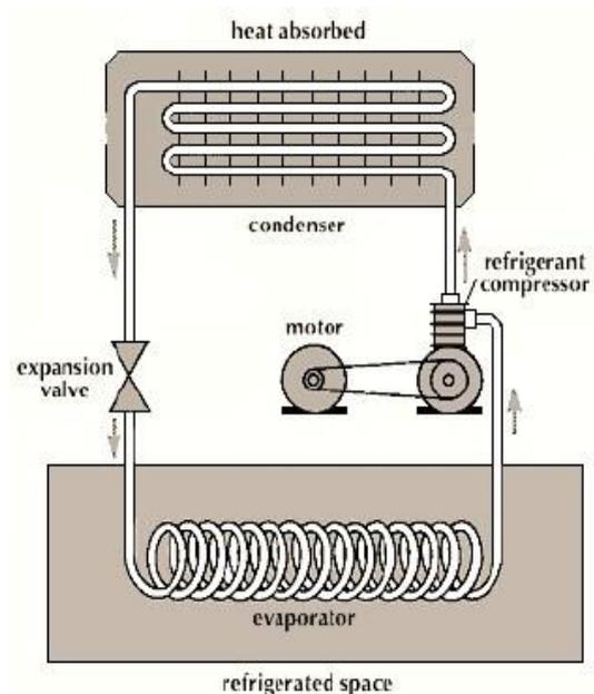
Fig. 1 Vapor Compression Refrigeration Cycle
