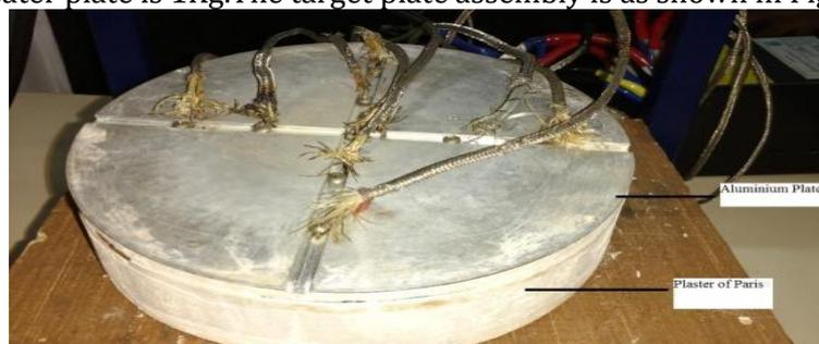
Fig 2b.Target Plate
