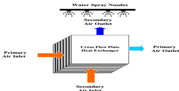
**Figure0 working principle of Indirect Evaporative Cooler [8]**
