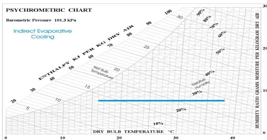
**Figure 2 Psychrometric Chart of Indirect Evaporative Cooler [5]**
