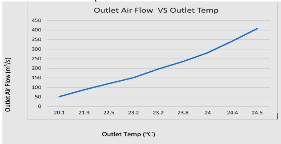
**Figure 4. Graph Outlet Flow vs Outlet Temp**
