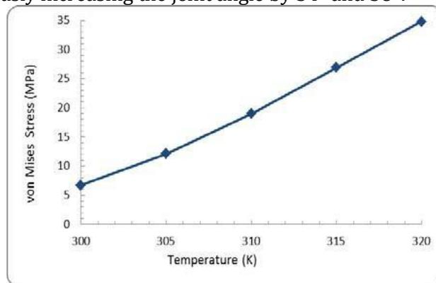
Figure 8: Stress - Temperature relation (load constant)
