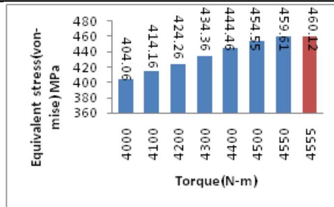
Figure 11: Equivalent stress in the universal joint at respective torque values
