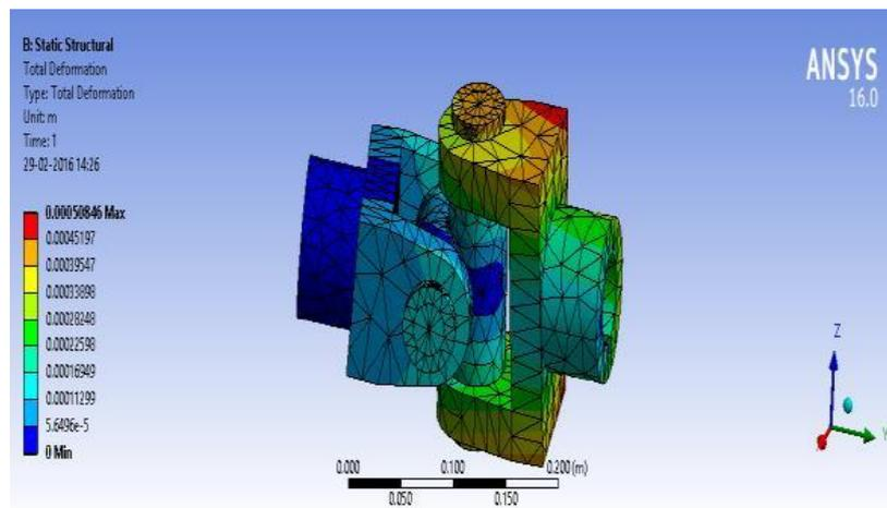
Figure 10: Total Deformation
