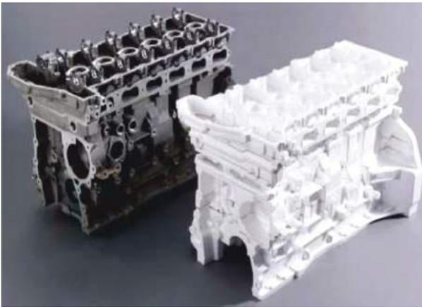
Fig 3 : Cylinder Block
