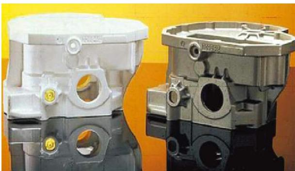
Fig 5: Trunk body casting and Foam pattern
