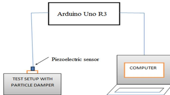
Fig 2: Proposed Schematic Experimental Test Set Up
