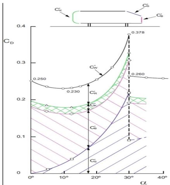
Figure 5: Diagram of the drag coefficient of Ahmed's base model
