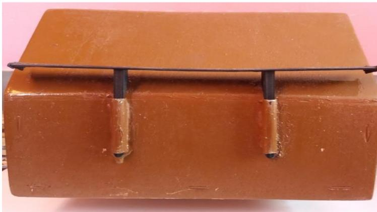
Figure 9: How the spoiler positions on the test model
