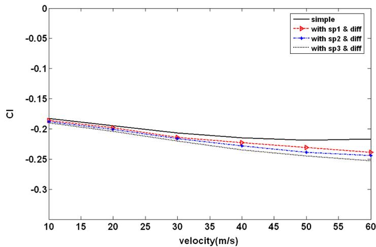
Figure 14: Changes of lift coefficients relative to speed
