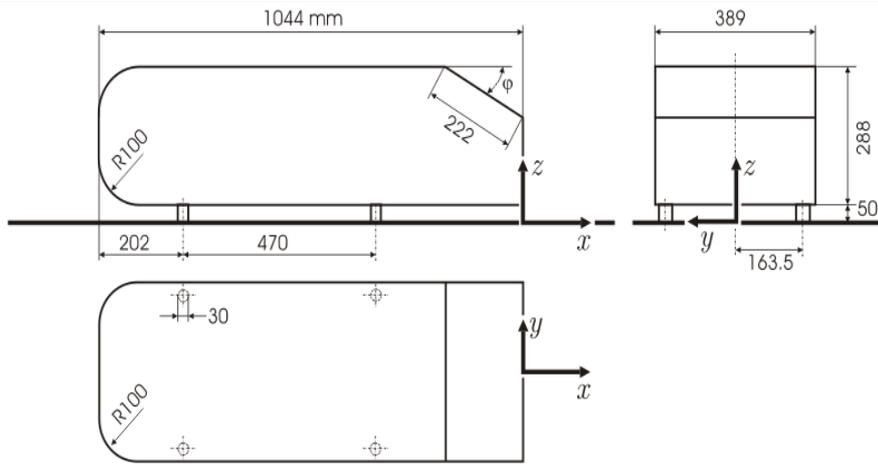
Figure 3: Characteristics and dimensions of Ahmed's model
