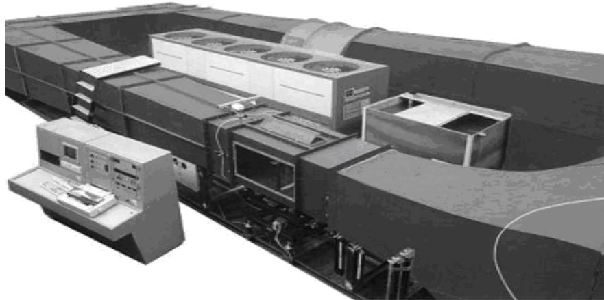
Figure 1: Subsonic wind tunnel of Aerospace Research Institution, Shiraz
