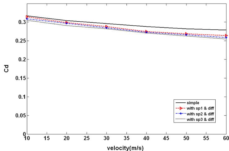
Figure 15: Changes in the drag coefficient relative to speed
