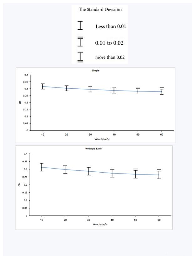
Figure 11: Diagram of determining the standard deviation of drag coefficient
