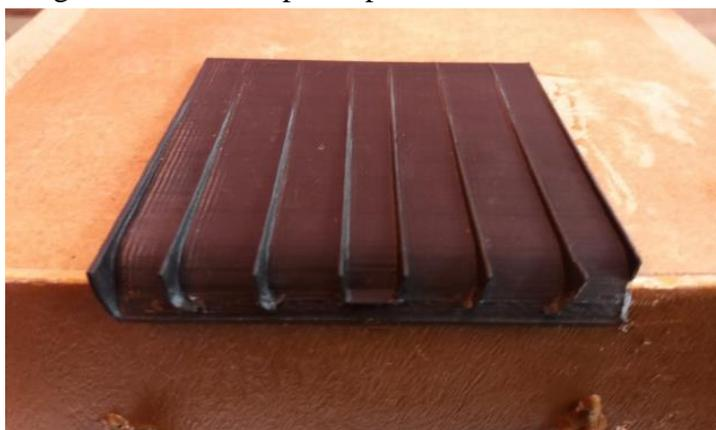
Figure 10: How the diffuser positions on the test model
