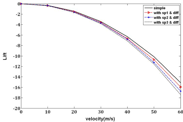
Figure 12: Changes of lift force relative to speed
