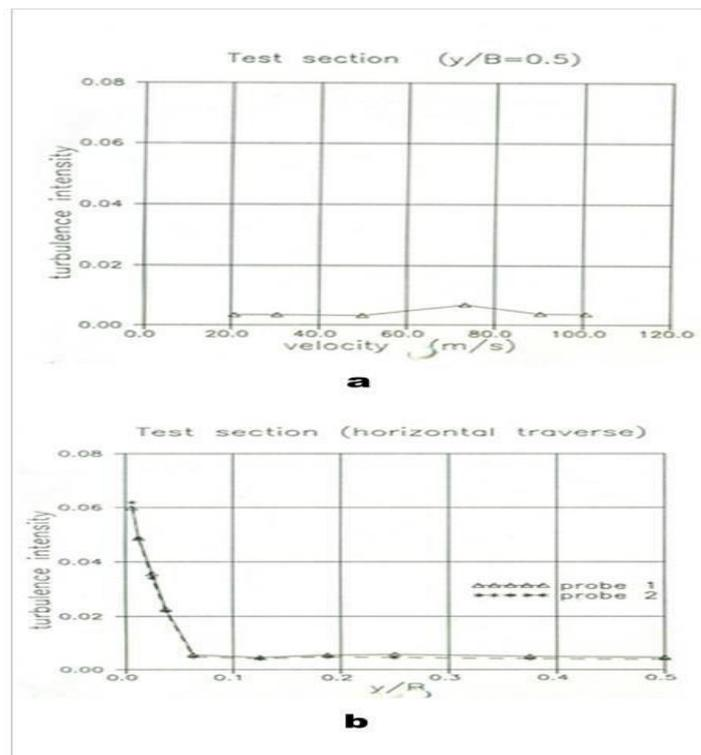
Figure 2: Changes of turbulence intensity in relation to the average speed in the center of the experiment section (a) and in relation to the distance from wall in the experiment section (b)
