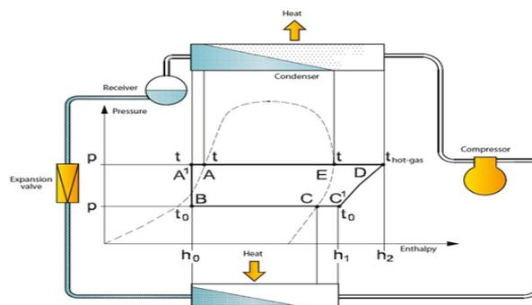
**Figure:-Combined Diagram VCR Cycle & P-H Diagram**
