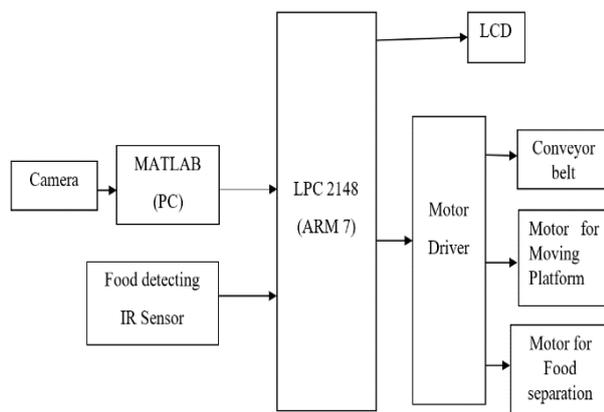
**Fig. 1.** Block diagram Of Automatic Fruit Sorting and Quality Analyzer
