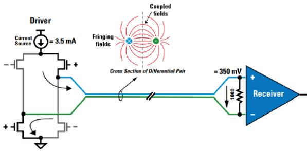
Fig-1: Low Voltage Differential Signaling [3]
