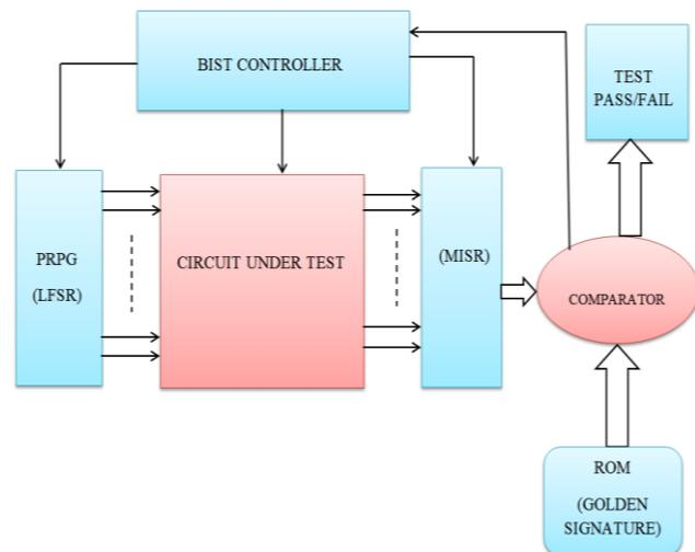
Fig.1 General Block diagram of logic BIST [4]
