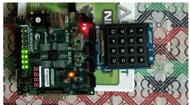
**Fig. 4** FPGA and keypad interfacing
