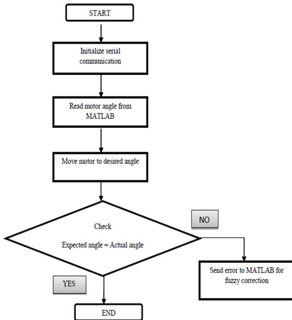
**Fig. 5** Flowchart of Microcontroller code
