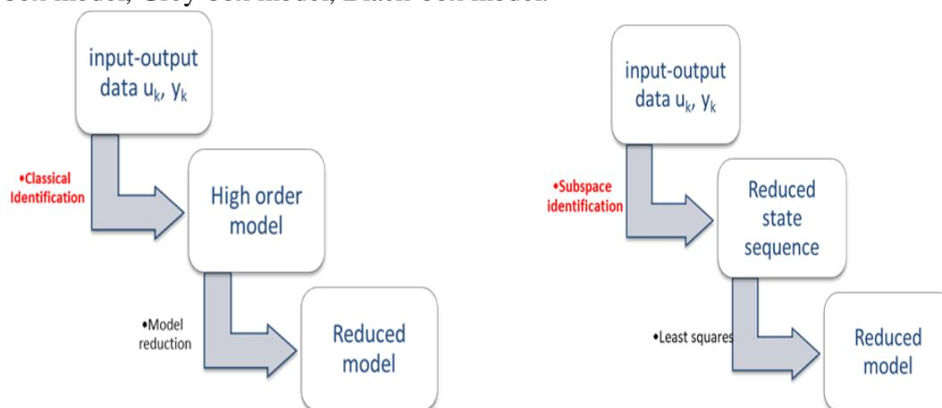
Figure 1. System Identification with Classical Identification and Subspace Identification
