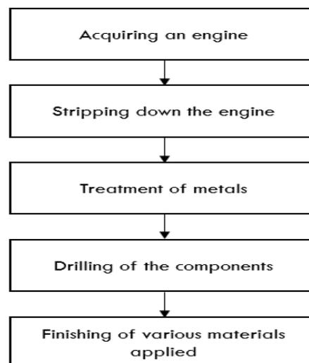
Process of upcycling engine table is as shown in the flow chart.
