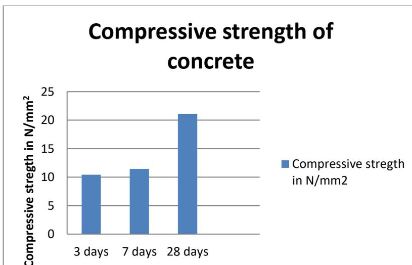
Figure.8.6 compressive strength of concrete with 30% replacement of Cement & Sand
