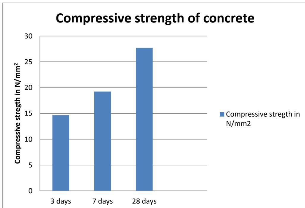
Figure.8.4 compressive strength of concrete with 20% replacement of Cement & Sand
