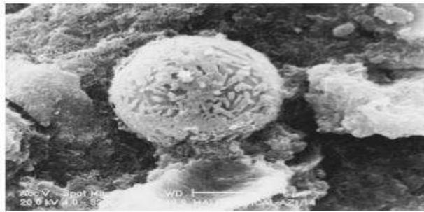
**Figure 4.3 Bottom Ash particle starting to react with Ca(OH)<sub>2</sub>**
