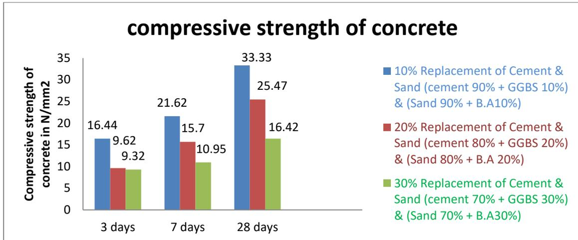
Figure 8.8 Compressive strength of concrete with different % replacements of Cement with GGBS & Sand
