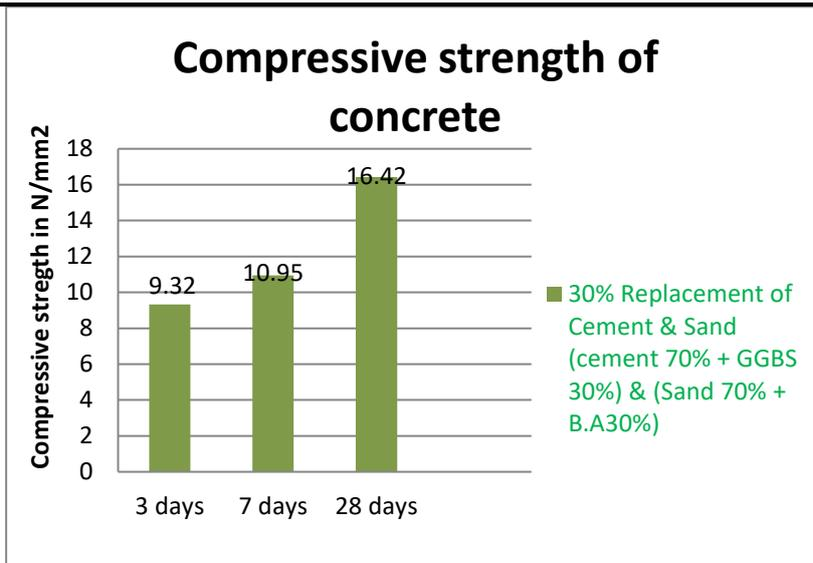
Figure 8.5 compressive strength of concrete with 30% replacement of Cement & Sand
