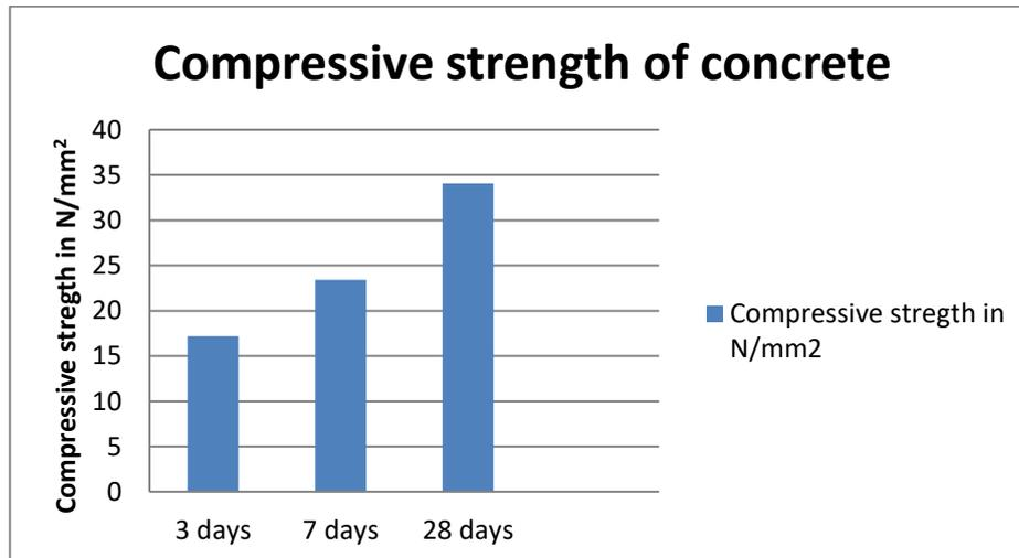
Figure.8.2 compressive strength of concrete with 10% replacement of Cement & Sand
