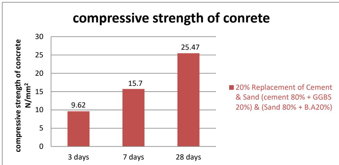
Figure 8.3 compressive strength of concrete with 20% replacement of Cement & Sand
