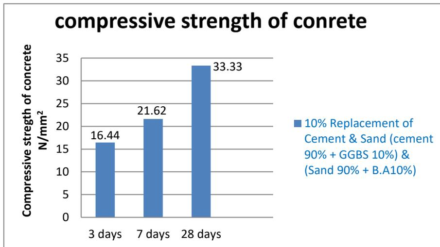
Figure 8.1 compressive strength of concrete with 10% replacement of Cement & Sand
