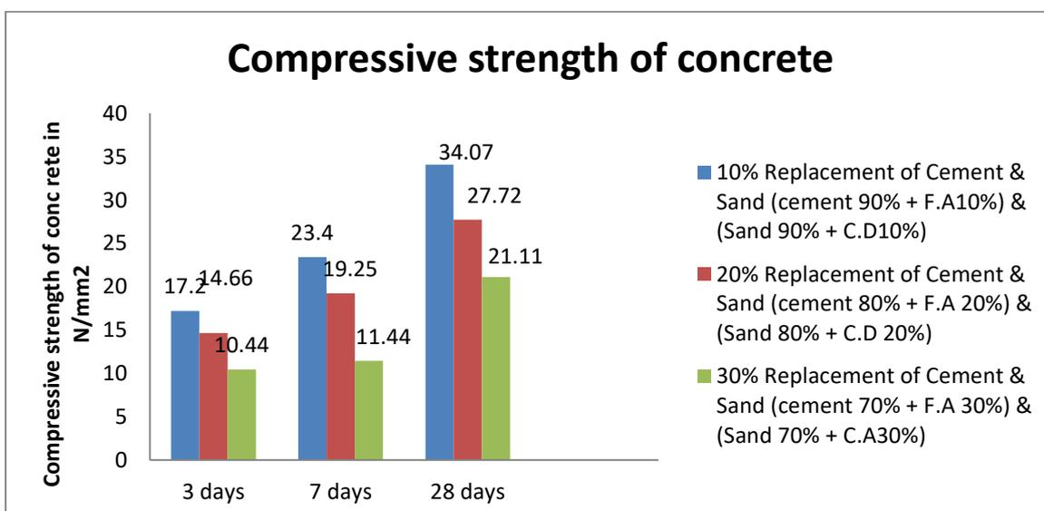
Figure.8.7 compressive strength of concrete for different % of replacement of cement with F.A and sand with C.D
