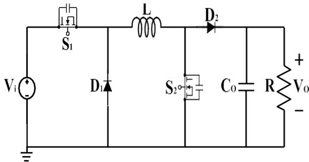
Fig.2. Circuit diagram of two switch buck-boost converter with DC source.
