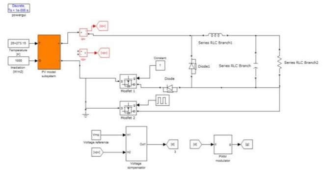
Fig.5 (b). Simulink model for boost mode.
