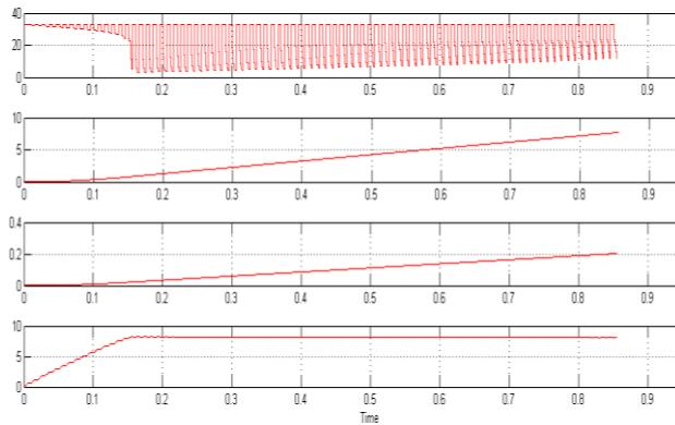
Fig.6 (a). Plot 1-Input voltage, Plot 2-Output voltage, Plot 3-Output current, Plot 4-Inductor current in buck mode operation.
