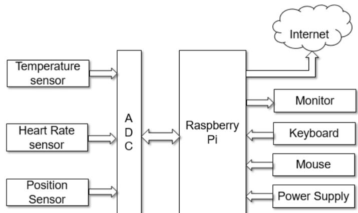
Fig. 1. Block diagram of Health Monitoring System using Raspberry Pi
