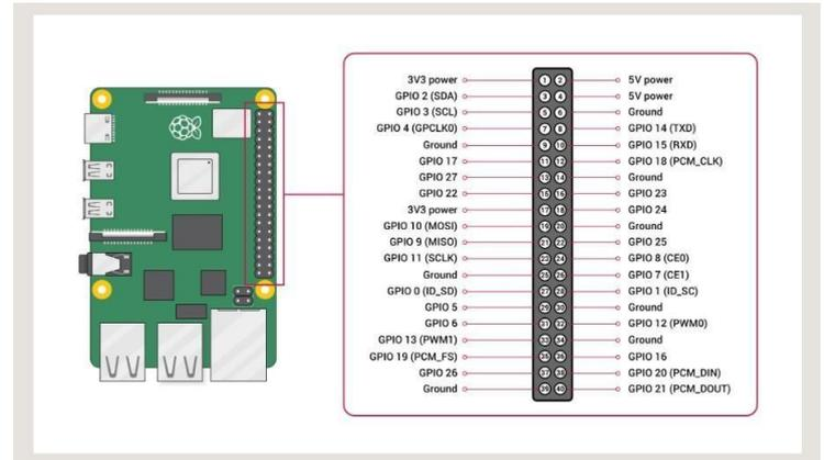
Fig. 3. Raspberry pi Pin diagram
