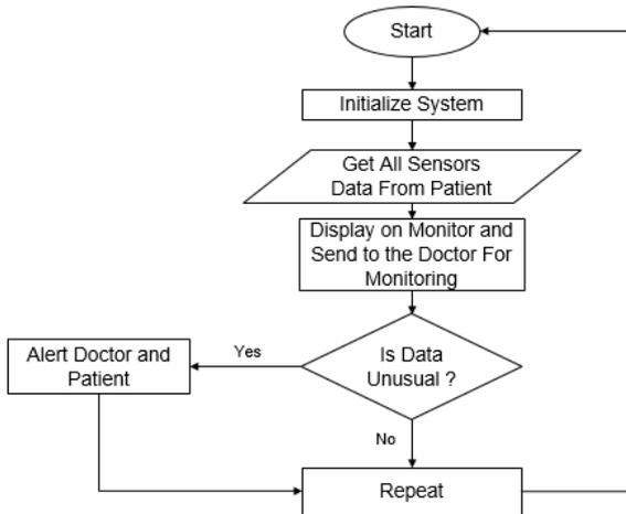
Fig. 2. Flow Diagram of Health Monitoring System using Raspberry Pi
