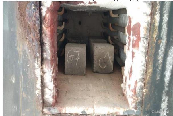
Fig. 2 Concrete Specimens kept in furnace for checking temperature effect
