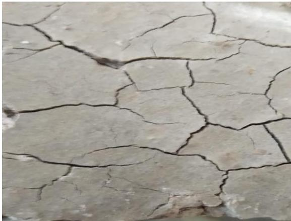
Fig. 3 Concrete surface cracks after exposed to 700<sup>0</sup>C
