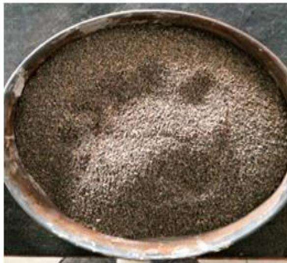
Fig.1 a. Recycled fine aggregate
