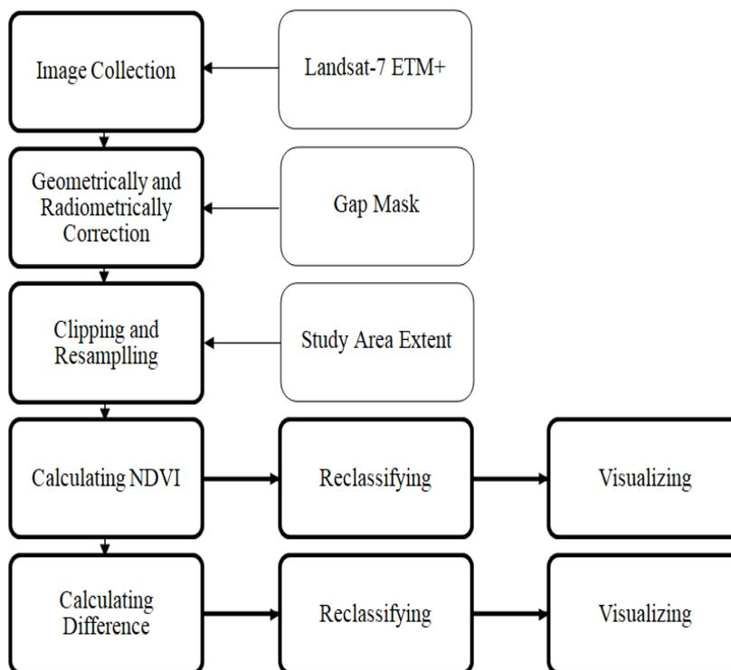
Figure 1: Flowchart of operation
