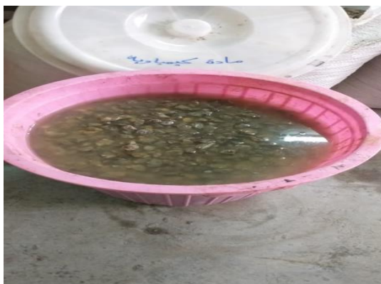
Fig. 2: Presoaking RCA in Sodium Metasilicate Pentahydrate Solution
