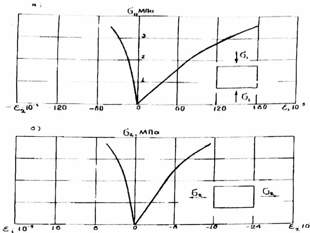
Fig. 1. The nature of the change in the relative deformations of non-autoclaved aerated concrete (on unmilled sand, IX series) during central compression-a and tension-b) (with the elimination of the effect of friction).
