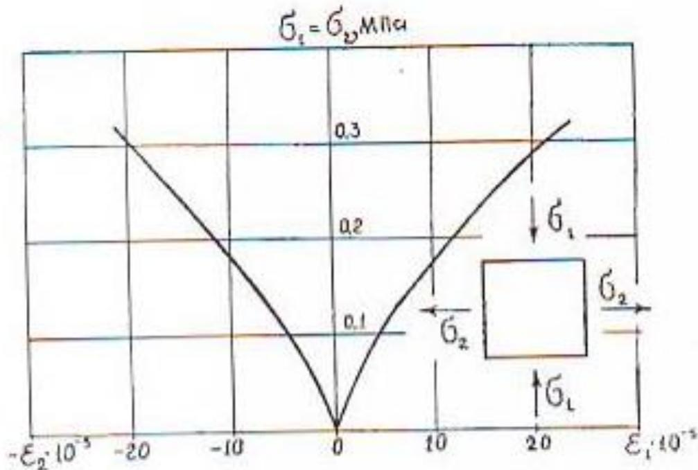
Fig. 2. Changes in the relative deformations of non-autoclaved aerated concrete under pure shear conditions.
