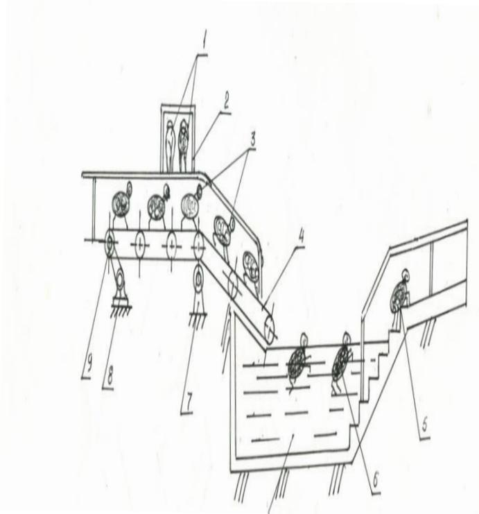
1 sheep in a cage; 2- iron cage; 3- sheep move along a conveyor; 5,6-sheep bathe in a bath; 7-support roller; 8-belt conveyor with a movable electric motor; 9-roller belt tension; 10-special chemical solution.
