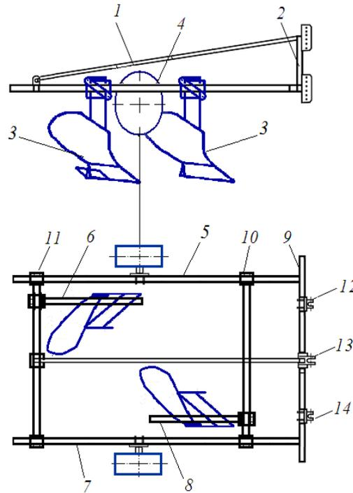
Figure 1. Design scheme of laboratory-field device: 1 - frame; 2 - hanging device; 3 - left and right bodies; 4 - base wheel; 5, 6, 7 and 8 - longitudinal beams; 9, 10, 11 - transverse beams; 12, 13 and 14 - brackets of the suspension device
