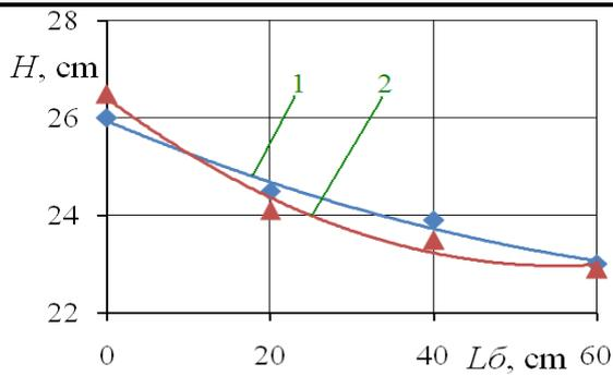
Figure 3. Depending on the height (H) of the ridge profile and the longitudinal distance ( $Lb$ ) between the bodies, the change in graphs 1 and 2, respectively, the operating speed is 6 and 9 km / h.
