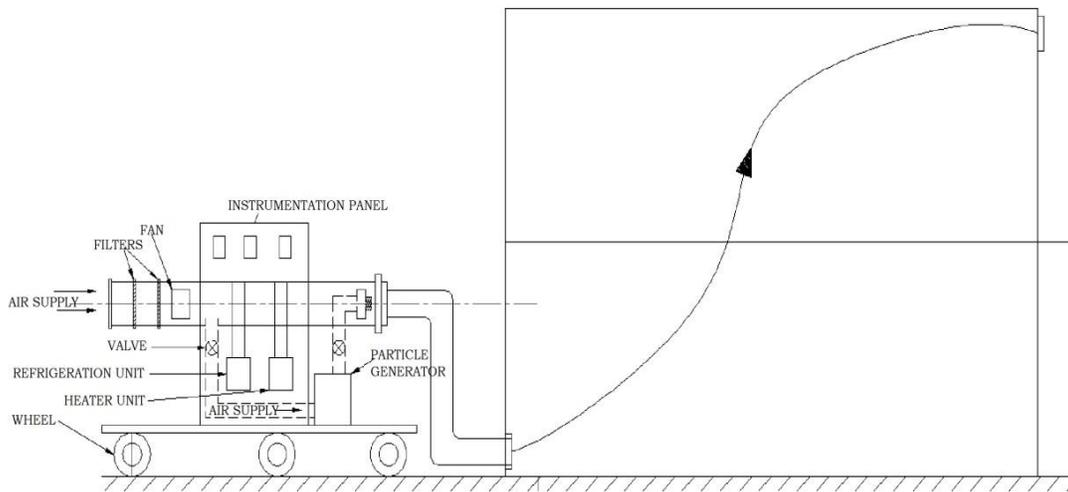
**Figure 2.1 Experimental Set-up for Displacement Ventilated Room**
