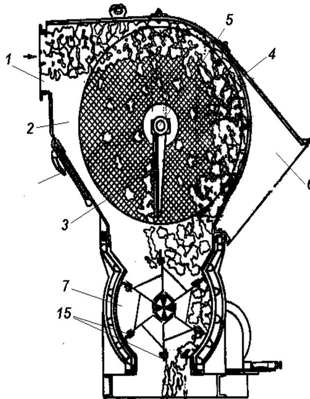
(Figure 2). Cross-sectional view of the CC-15A separator
