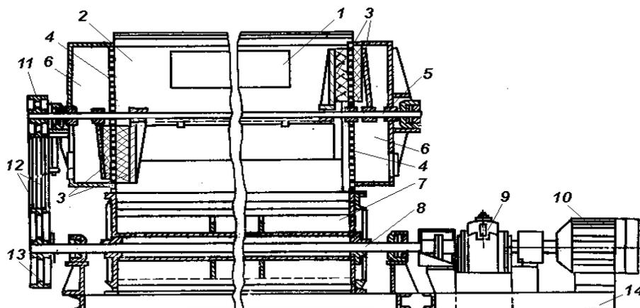
(Figure 1). Log cross-section surface of CC-15A separator.
